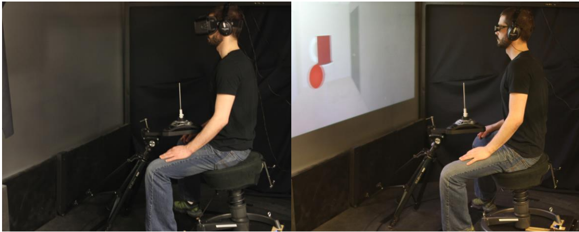
Figure 3.12. HMD with joystick (left) & 3D projection screen with joystick (right)
