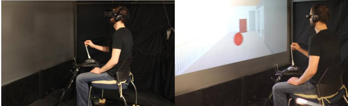
Figure 3.12. HMD with joystick (left) & 3D projection screen with joystick (right)
