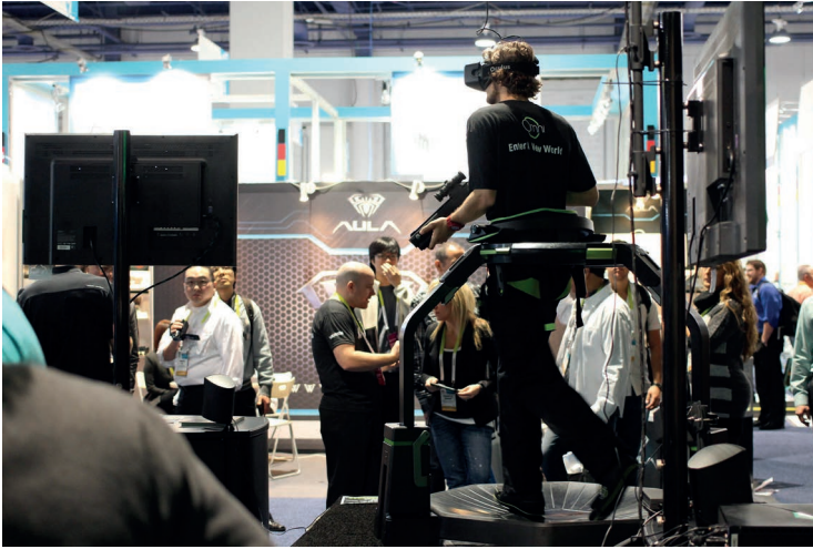
(a) A passive omnidirectional treadmill supports the user's centre of mass. Maurizio Pesce, CCBY2.0
