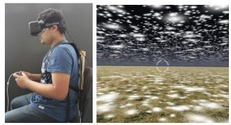
Figure 1: Left: Participants wore a HMD (Oculus Rift DK2) and custommade backpack carrying the inclination sensor (PhidgetSpatial 1042). Right: Visual stimuli of the virtual environment designed to provide strong optic flow but no landmarks.
