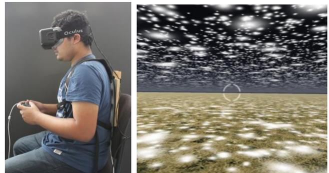
Figure 1: Left: Participants wore a HMD (Oculus Rift DK2) and custom-made backpack carrying the inclination sensor (PhidgetSpatial 1042). Right: Visual stimuli of the virtual environment designed to provide strong optic flow but no landmarks.
