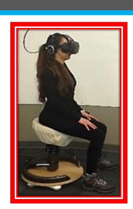
**NaviChair** User sits on a seat/stand stool (Swopper<sup>TM</sup>) mounted on top of a Wii Balance board force plate, and controls forward/ backward and sideways translation by shifting their weight toward the corresponding direction.
