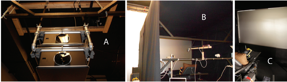
Figure 2-1: (A) The IN5504 projector pair behind the tent. Note the polarizer panels mounted in front of the projector lenses. (B) The tent installation surrounding the screen and viewer. (C) A shot from behind the seat.
