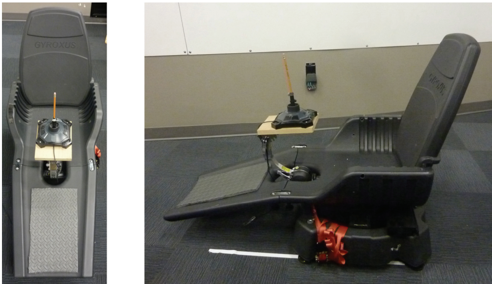
Figure 2-8: (Left) completely assembled product with joystick replacement. Note the adjustable backrest and removable, suspended footrest. (Right) Left view of the gyroxus gaming chair. Note the box underneath the seating surface resting on crossed metal ropes and the blocks/tie-strap to keep the seating surface stable during non-physical motion.
