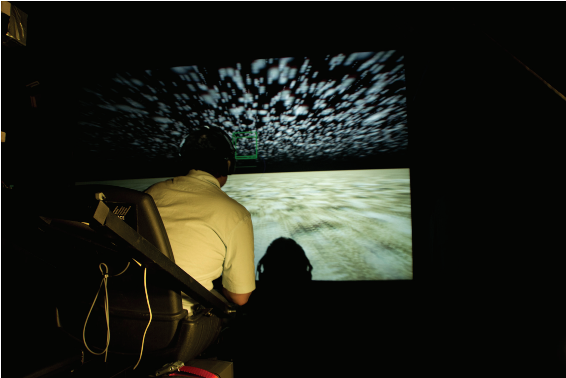
Figure 2-9: The Gyroxus gaming chair affords leaning to control velocity and direction of VR locomotion.
