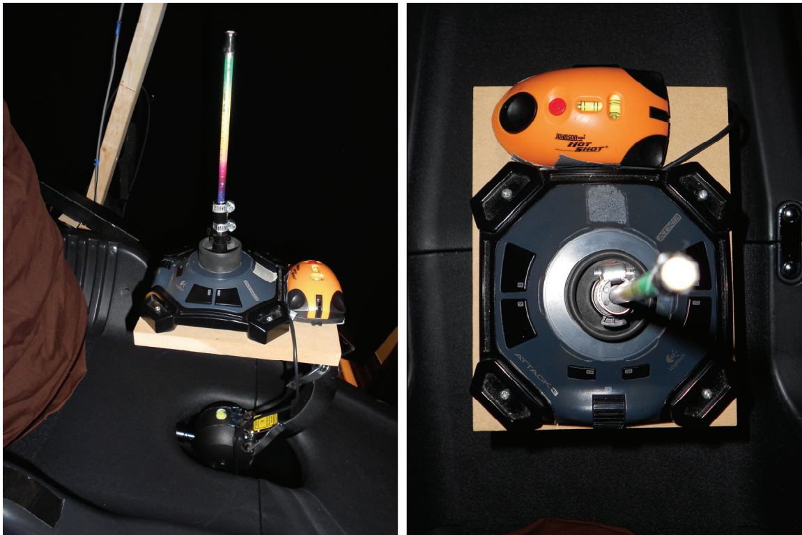
Figure 2-12: Left: Joystick and level gauge (orange device) mounted on the Gyroxus. Right: Top-down view on the Joystick, similarly as to what the participant would see while seated looking down on the joystick. Note the black buttons on the joystick base.
