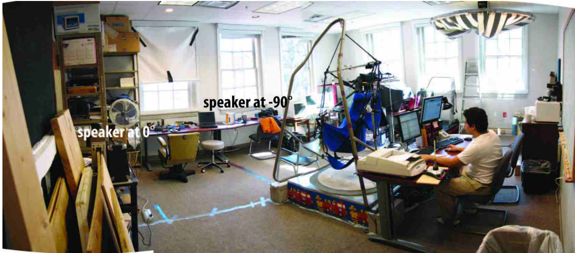
Figure 1: Roundshot photograph of the lab space and the experimental setup showing the hammock chair, the experimenter setup, and the two speakers, one in front of the chair and participant's default orientation at 0^\circ (left, Guitar amplifier), the other one to the right of the chair at -90^\circ .
