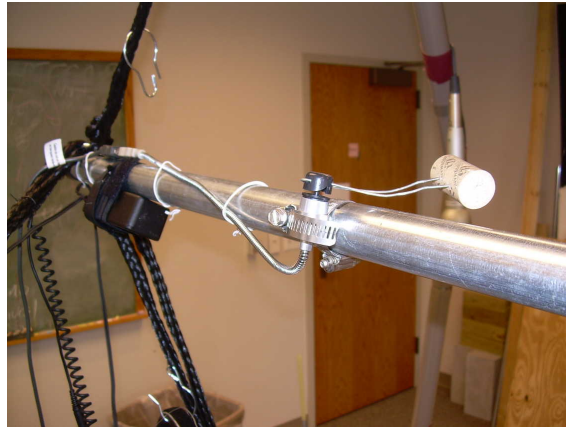
Figure 5: A USB fan was modified to act as an excenter motor that provided a barely noticeable jitter of the hammock chair. The picture shows the wire, which connects the cork with the motor which in turn is connected to the crossbar. A tubing extends beneath the motor, guiding the USB cables safely to an extension cord, which was connected to the USB port of the left monitor on the desk. It was plugged/unplugged to switch on/off the motor. The battery module of the binaural microphones can be seen beneath the USB connection of the motor, mounted on the crossbar using Velcro.
