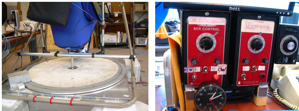
Figure 3: Left: Experimental setup, as seen from the back. The u-bar (70 centimeters in width and height) beneath the chair holds it in position and relays the rotation of the rod extending from the platform to the chair. As shown in the picture, the u-bar can be fixed through a beam 140 centimeters in length attached to the support bars on the far sides for walking conditions. The black laptop-bag is hanging from the back of the chair. Two strong wires from the left and right connect the bag to the u-bar, preventing it from moving extensively and hitting the participant's back. Right: Analog control unit that could be used to rotate the chair and platform independently. The white unit next to the yellow envelope is the access point (Netgear WGT 624v3) for wireless communication between the laptop and desktop computers. The clock and metronome (mounted on the right controller) can be optionally used for timing purposes.
