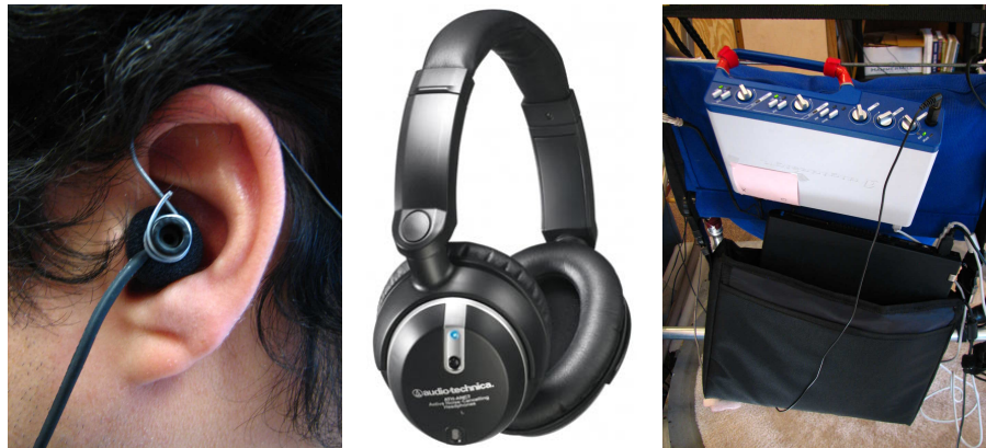
Figure 6: Left: Core Sound Binaural Microphone that was mounted right outside the ear canal for binaural recordings. Middle: Audiotechnica AT-7ANC active noise canceling headphones used for playback. Right: DigiDesign MBOX2 audio-interface used for high-quality recording and display. The laptop computer mounted in the bag is visible beneath.
