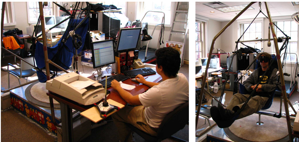
Figure 2: Experimental setup, as seen from the experimenter's view (left) and the front with a participant seated in it with his feet suspended in the footrest (right). The left picture shows the computer interfaces. The screen to the experimenter's left displayed the data sheet in which the conditions and responses were accessible. The right screen displayed the ProTools audio suite. The chair can swing slightly forwards and backwards. During trials, the participant's knees are in a 90^\circ angle, as illustrated in Figure 4. In the top right part, a microphone (Realistic 331070B) is hanging from the mount. It can be used optionally for session recordings.
