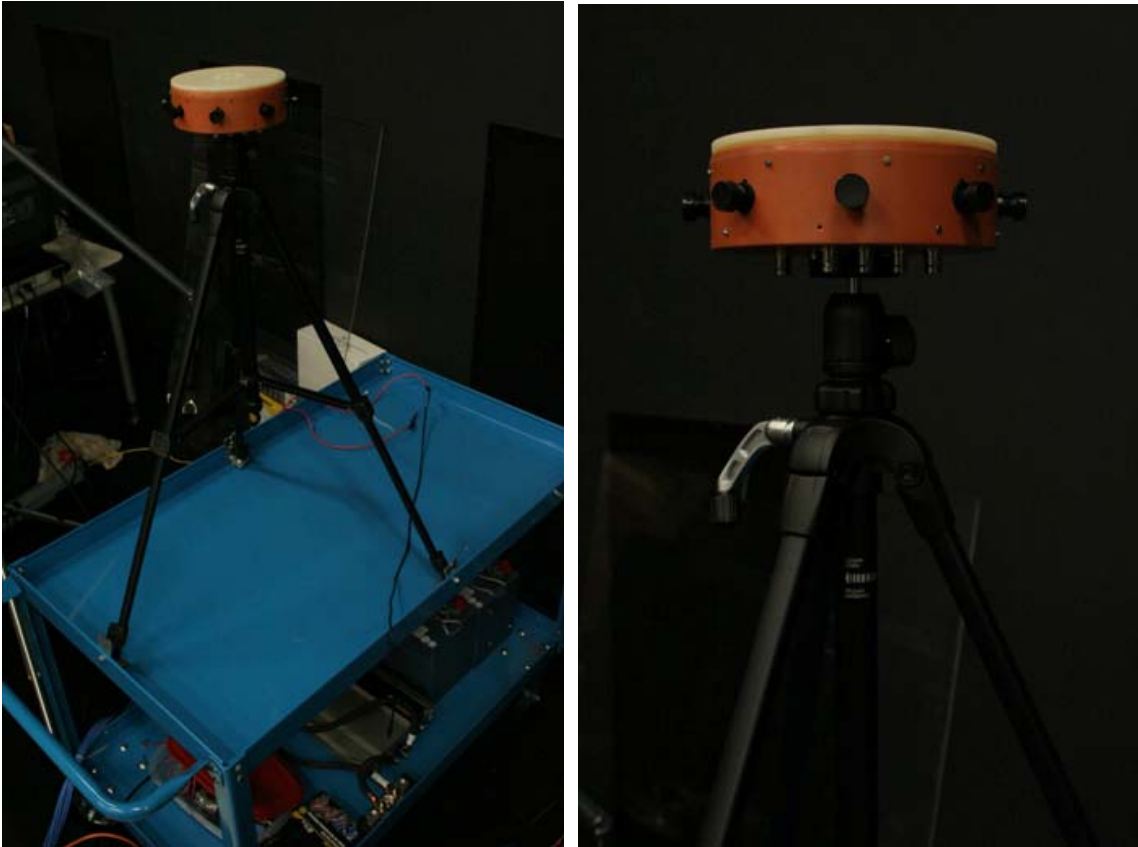
Figure 1: Panoramic video capturing system. It includes 8 cameras mounted on a trolley which carries a PC and batteries for powering the cameras and the PC.
