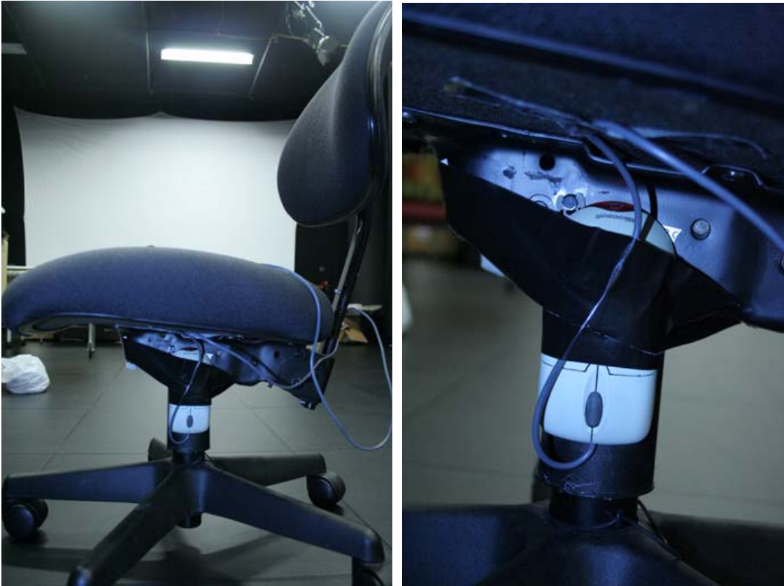
Figure 2: Interactive chair interface for supporting body-based rotations in the panoramic video. The chair is a regular office chair which is modified by attaching an optical mouse to its rotating pivot. The mouse detects user's rotations in 360 degrees and the display system displays the corresponding part of the panoramic view.
