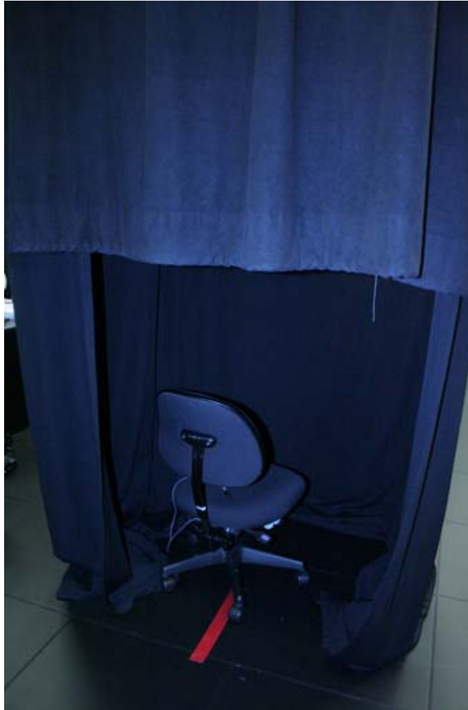
Figure 6: The immersive platform for running the experiments in the SIAT Virtual Reality lab. It contains the interactive chair in a dark space disconnected from the outside distractions by black drapes.
