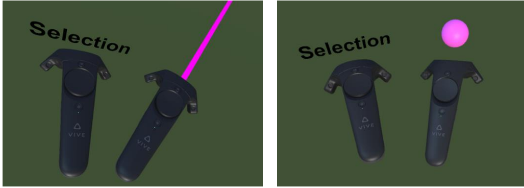
Figure 2: Appearance of the VR controllers in the 2 selection modes. Left: raycasting. Right: virtual hand.
