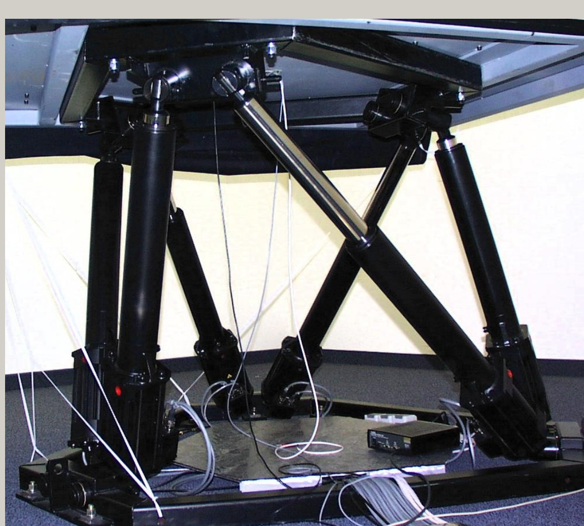
Fig. 2: Electric 6 degrees of freedom motion platform (Motionbase Maxcure)
