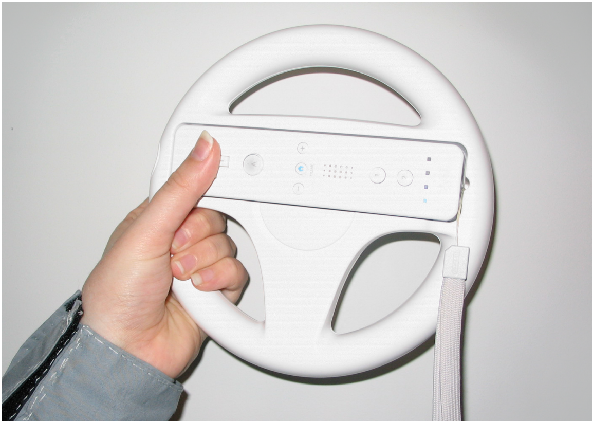
Figure 7 The Wiimote is embedded in the Wii Wheel, which is held like a steering wheel.
