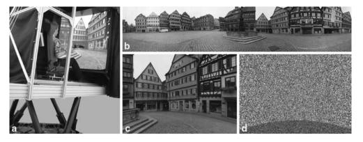
**Fig. 1 a** Participant seated in front of a curved projection screen displaying a view of the Tübingen market place. The whole setup is mounted on a motion platform. **b** Visual stimuli used in the FULL SCENE condition were generated by wrapping a  $360^{\circ}$  panoramic image ( $4,096 \times 1,024$  pixel) of a natural scene (the market place of the town Tübingen in southern Germany) onto a cylinder. **c** The rendering viewpoint was centered in the cylinder,
