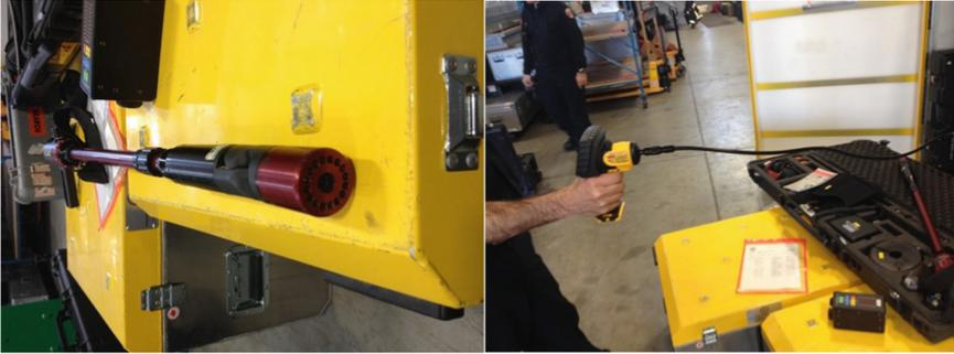
**Fig. 5.** Cameras. The left camera is designed specifically for USAR. The right camera is normally used in construction.
